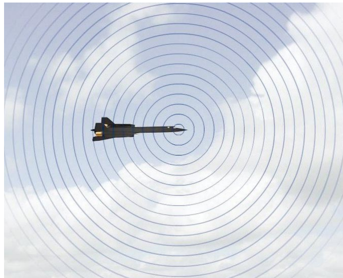
Figure 4.6 An illustration showing pressure waves emanating from a theoretically stationary aeroplane
