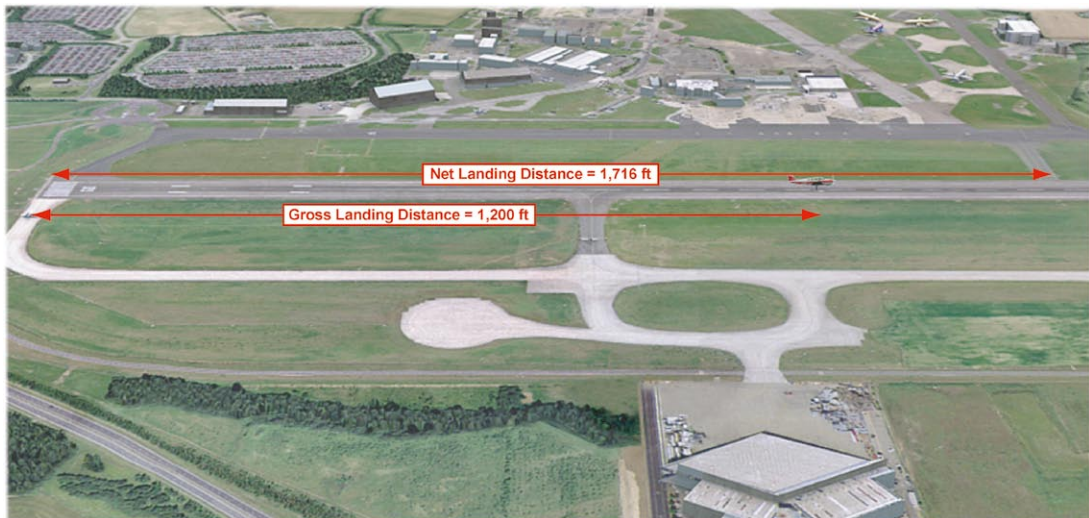
Figure 9.2 The obtain the minimum length of runway required, multiply the gross landing distance by 1.43
