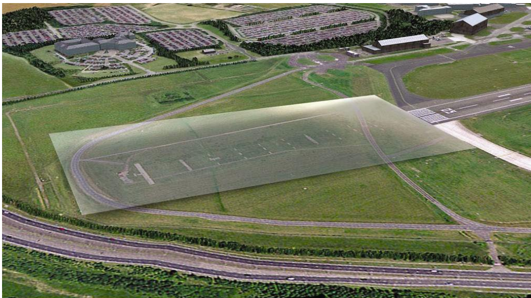
Figure 2.1 Clearways extend from the end of the runway with an upward slope not exceeding 1.25%, above which no object or terrain protrudes.
