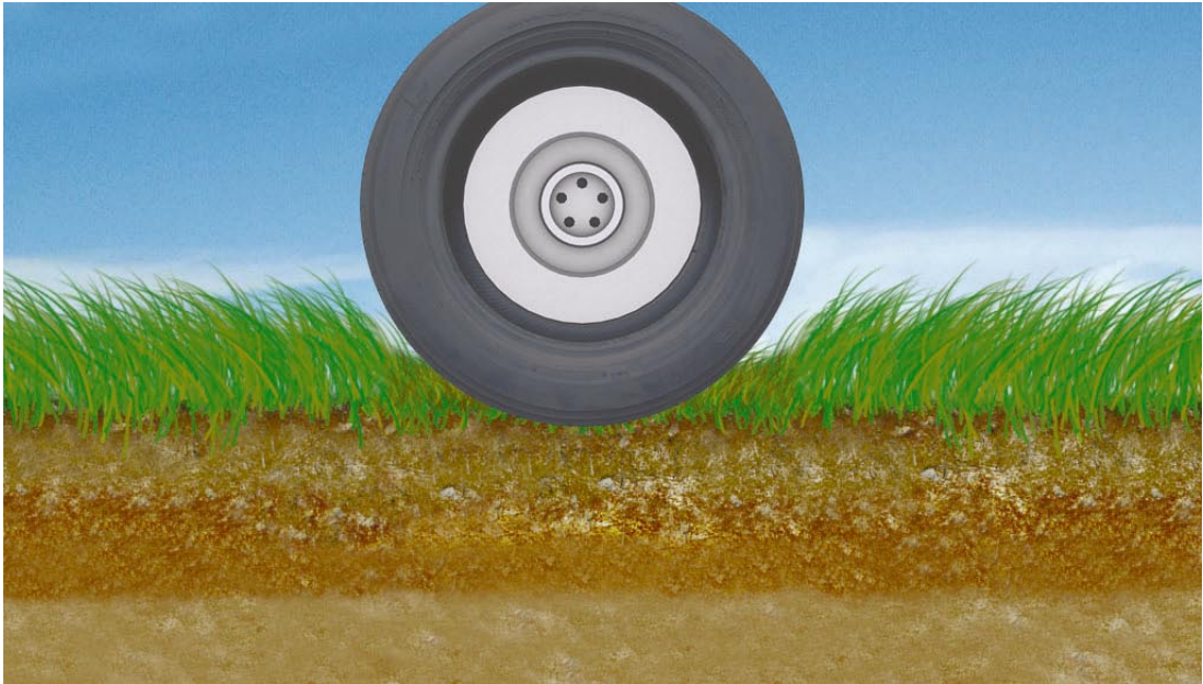
Figure 5.6 An illustration showing that for the wheel to advance grass must be pushed out of the way
