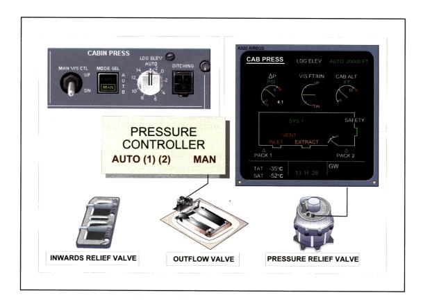
Figure 2.3. Electronic Pressurisation Control
