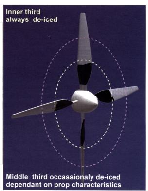
Figure 1.16. Propeller Icing System.
