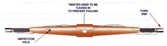
Figure 1.6. Wire Locked Turnbuckle
