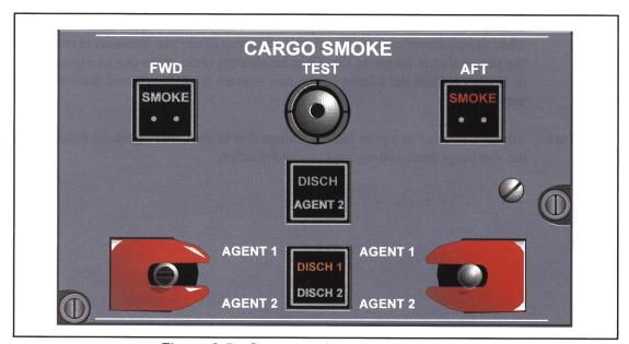
Figure 3.5. Cargo smoke detection (Airbus)
