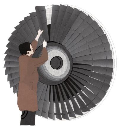
Figure 3.8. A High Ratio By-Pass Engine Low Pressure Compressor or Fan.
