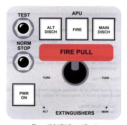
Figure 13.3 APU Control Panel
