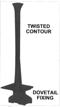
Figure 3.6. A Typical Compressor Rotor Blade
